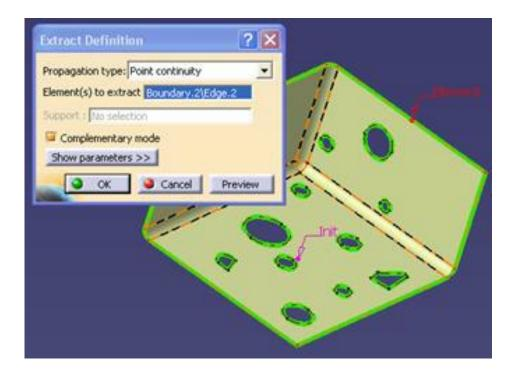
Create Boundary for the surface using boundary command. Select the full surface and press OK.
